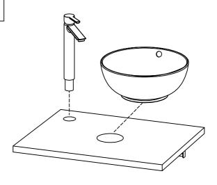
FIT THE BASIN WASTE, MAKING SURE THERE'S A GOOD SEAL. FIT ANY BRASSWARE AND CONNECTIONS IF REQUIRED AT THIS POINT. APPLY A BEAD OF SILICONE AROUND THE BASE OF THE BASIN THAT WILL BE IN CONTACT WITH THE WORKTOP. PLACE THE BASIN IN POSITION ON THE WORK SURFACE AND PRESS DOWN TO MAKE A SEAL. CLEAN OFF ANY EXCESS SEALANT
