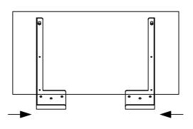
INSET SUPPORT BRACKETS FROM EACH EDGE TO REDUCE VISIBILITY ONCE INSTALLED.
